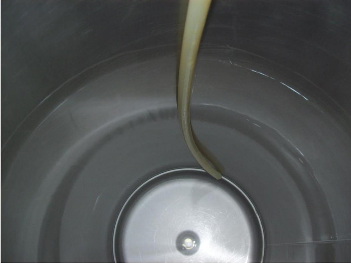
First installation step is to install the silicone tube onto the **out** port dip tube. Slide the tubing onto the dip tube at least 3/8". With a gentle tug, the tubing should stay put, if not, remove the tubing and dry the dip tube with a clean cloth. As you can see, the natural curvature of the hose is pointing towards the sidewall. This is **not** what you want. Rotate the tubing on the dip tube until it is positioned as seen in the next photo.
